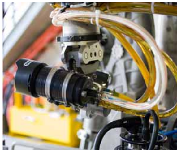
Ocean ProHD Camera on an Oceaneering Hydra ® Maxximum ROV
