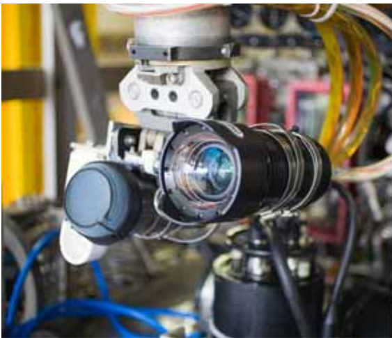
Ocean ProHD Camera on an Oceaneering Hydra ® Maxximum ROV
